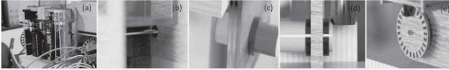
**Figure 2.** Electronic and mechanical components of our experimental device. (a) Arduino board. (b) Steel shaft. (c) Laser sensor at the top of the conducting tube. (d) Laser sensor at the bottom of the conducting tube. (e) Encoder and wheel used to measure the velocity of the falling magnet.
